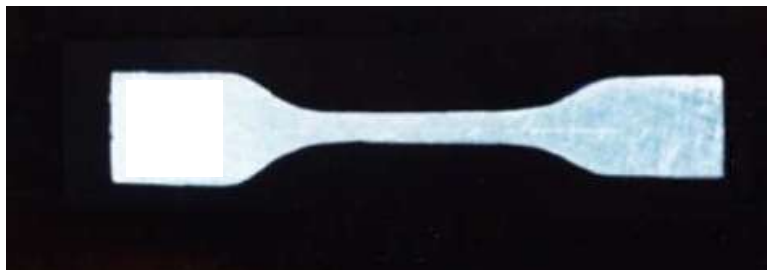
Figure (1): -Metal pattern for tensile bond strength.
