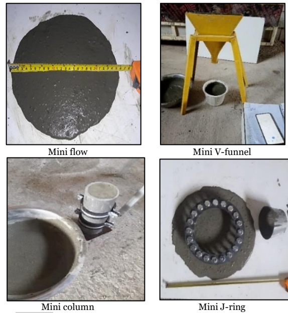
Fig. 3 Testing of the self-compacting mixture.
