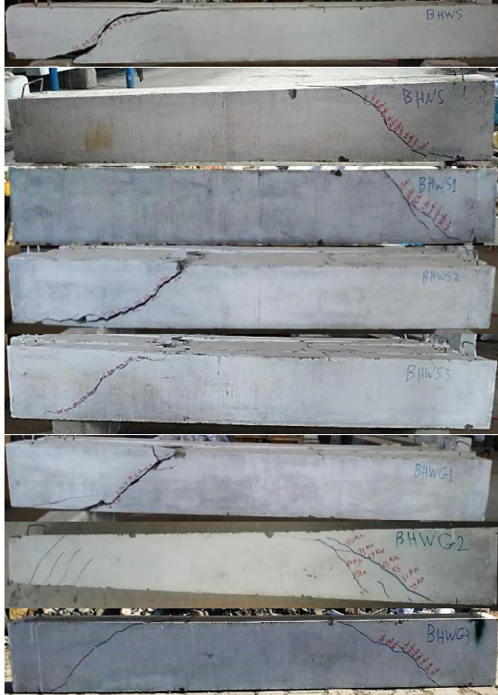
Fig. 9 Failure of shear ferrocement beam reinforced using steel and glass mesh.
