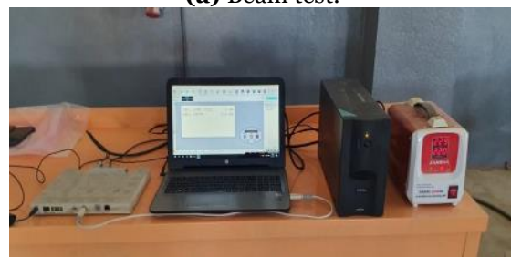
(b) Data logger to monitor the load and deflection.
