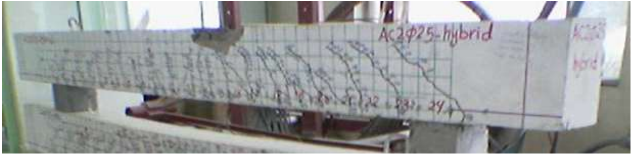
(a): Experimental Crack Patterns
