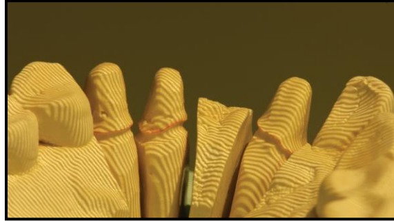
Figure (4): White light projector pattern by optical scanner (20)
