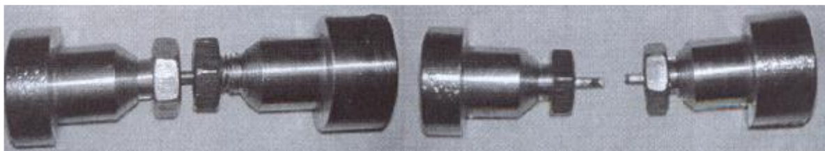
Figure-7: A: The grips holding the tensile specimen before testing. B: The grips holding the tensile specimen after testing (after rapture).
