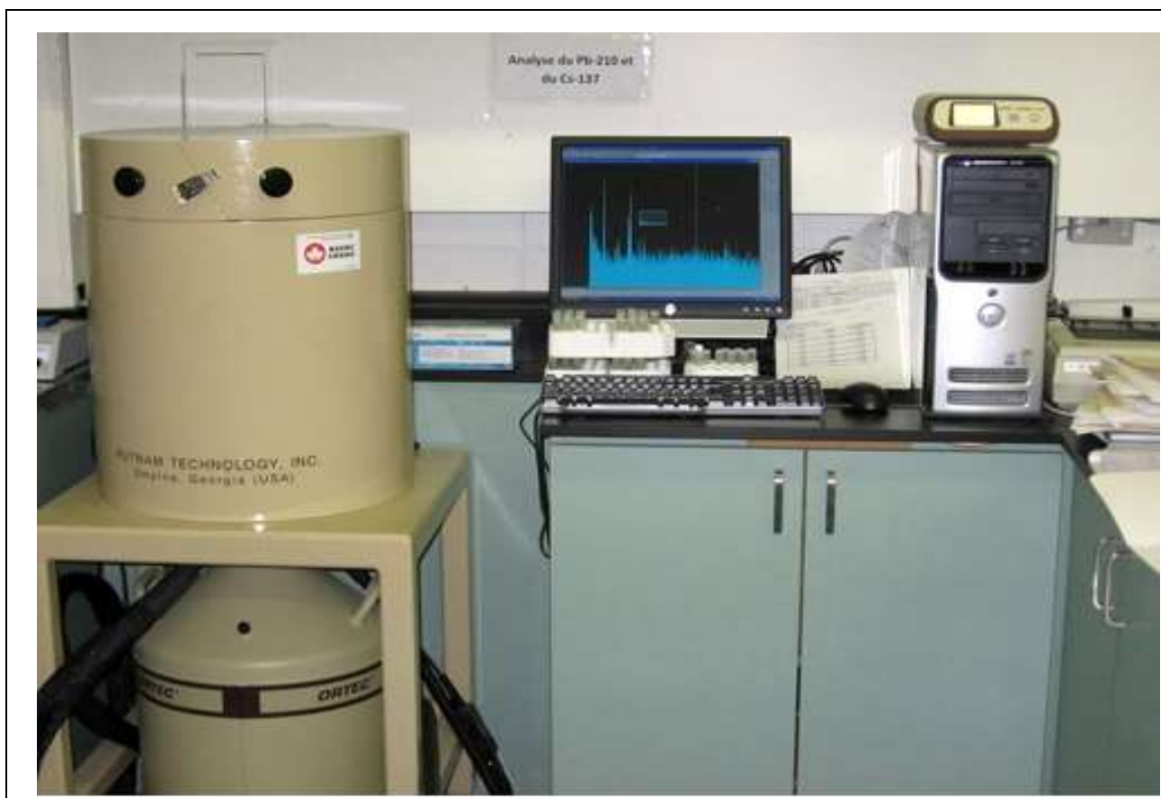
Fig(1) HPGe system for the counting of radionuclides
