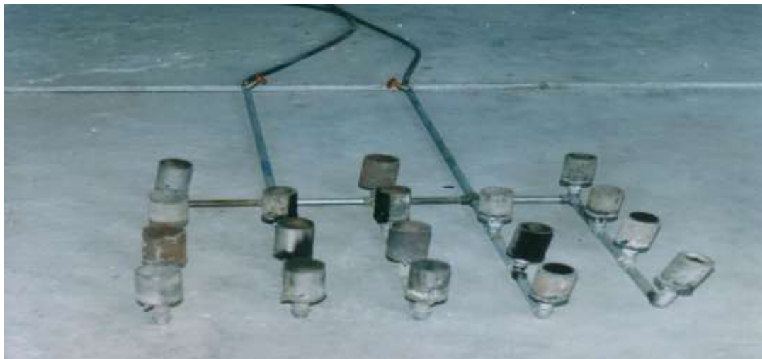
Figure (2) the network of burners
