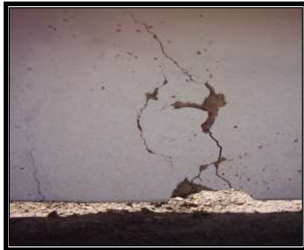
a. First crack appeared at 26% of the total beam length measured from the support
