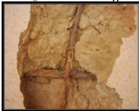
c. Final crack appeared at 26% of the total beam length measured from the support
