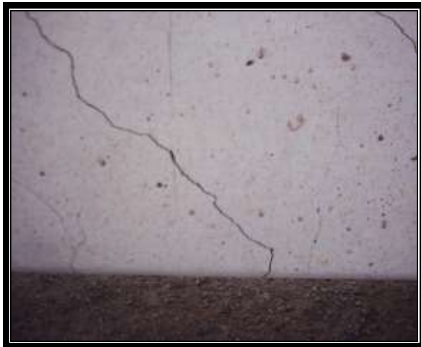
a. First crack appeared at 26% of the total beam length measured from the support
