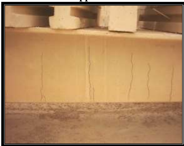
c. Final crack appeared at 26% of the total beam length measured from the support
