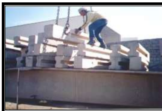
Fig. (4) General test setup for the tested non-prismatic beams [3]
