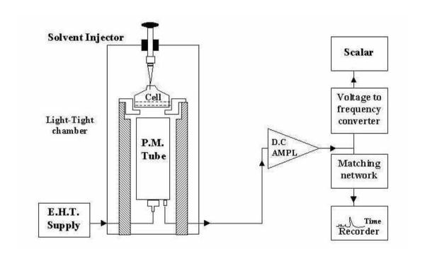
Figure 1. The lyoluminescence reader
