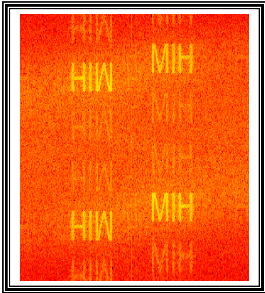
Fig(5): Digital reconstruction image of a hologram with random phase.
