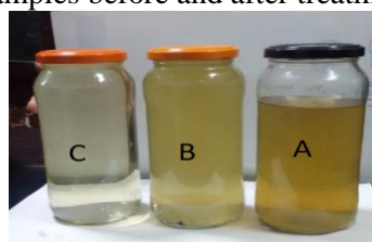
Figure 4. Changes in color and turbidity of greywater samples, A: Raw greywater sample; B: Same greywater after treatment in an anaerobic vessel; C: The same greywater after treatment in Aerobic vessel.
