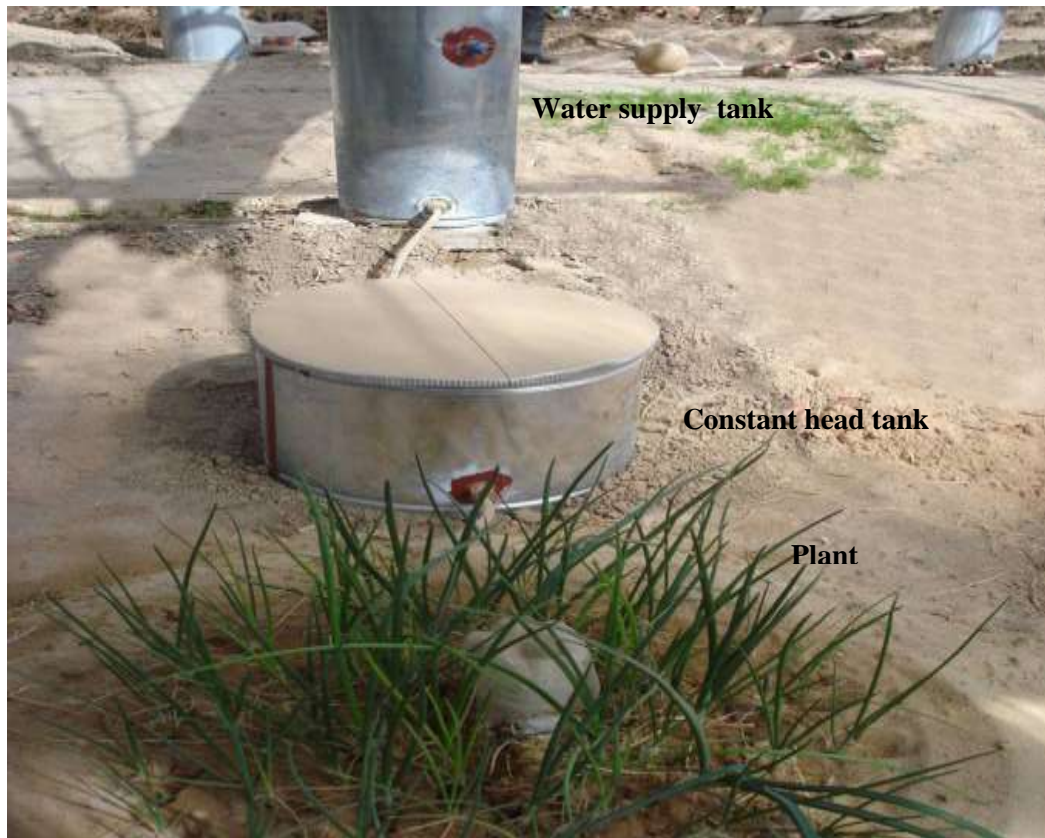
Figure (3). Asnapshot showing buried ceramic pot with agriculture.
