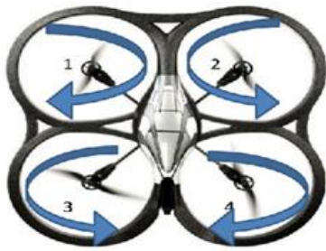
Figure 2 Rotation of the four motors
