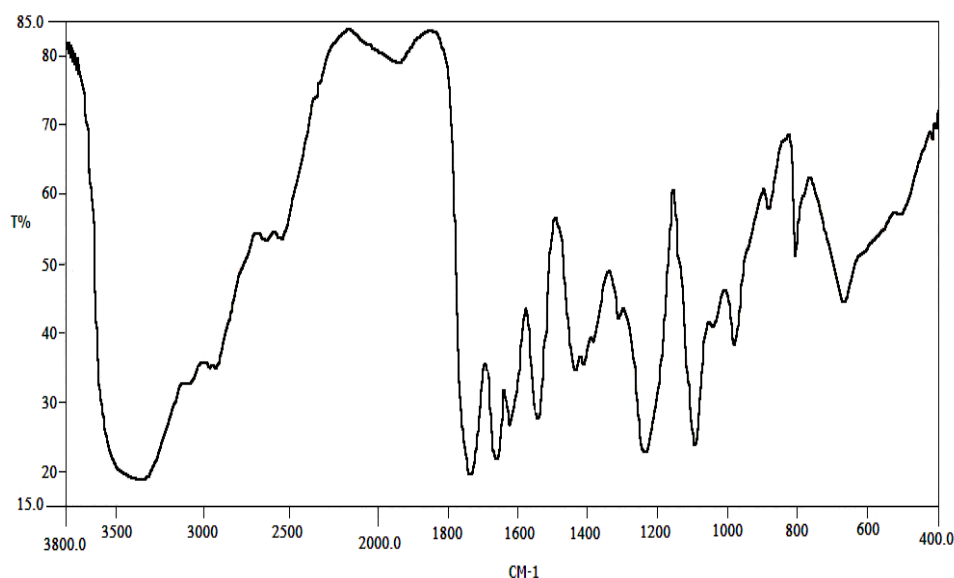
Figure 1. IR spectrum of acrylamide-N-methylene glycolic acid (AA-N-MGA).
