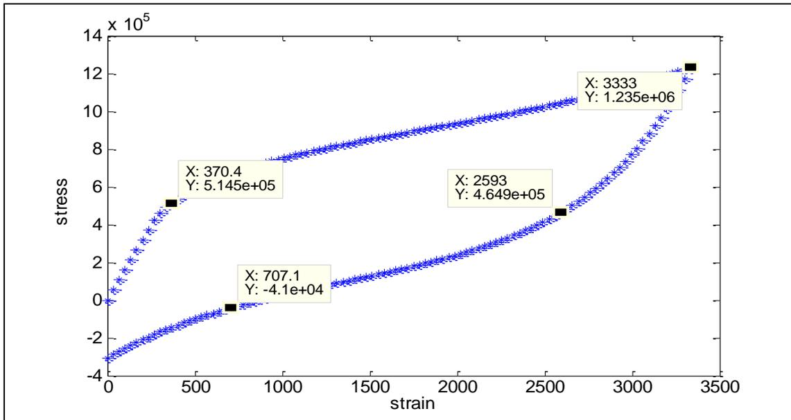
**Figure 6: Deformation-spring force hysteresis loop at 5°C.**
