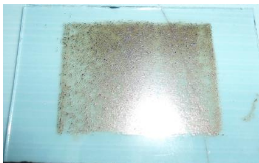
Figure 6. Shows the coated carbon nanotubes on ITO glass (counter electrode).
