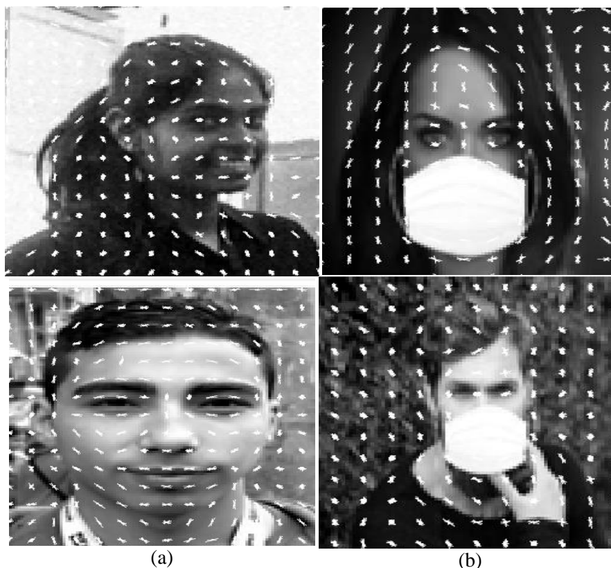
Figure 4. Illustrating the effect of HOG on (a) the non-mask face, (b) the masked face.
