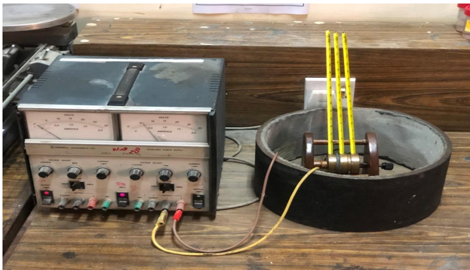
Figure 3. shows thermal conductivity measurement (Lee's Disc)
