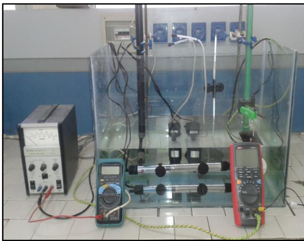
Fig. 2 Photo of the Installed ICCP System.
