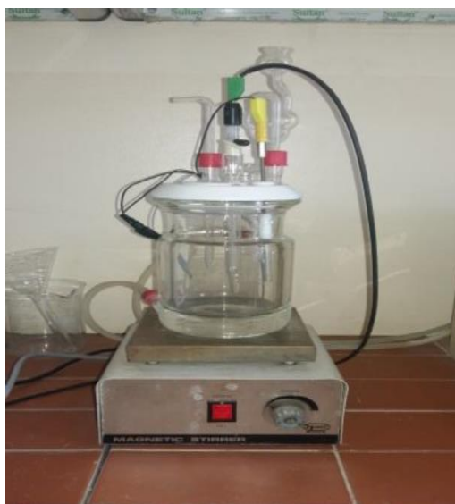
Figure 2. Set up the corrosion cell and three electrodes
