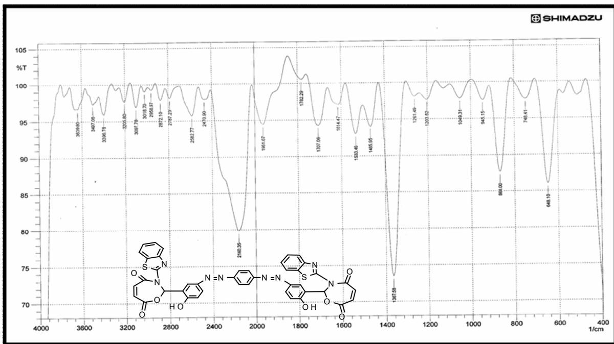
Fig.9:FT-IR spectrum of compound [9]
