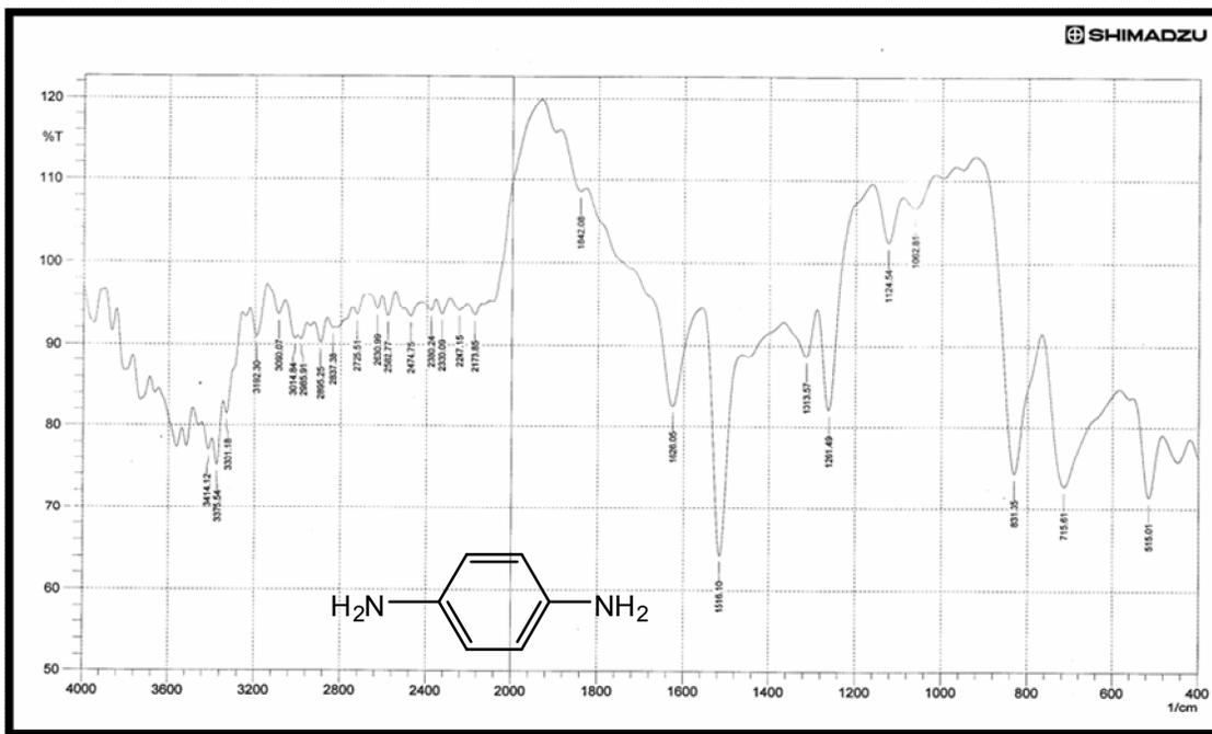
Fig. 1:FT-IR spectrum of compound [1]
