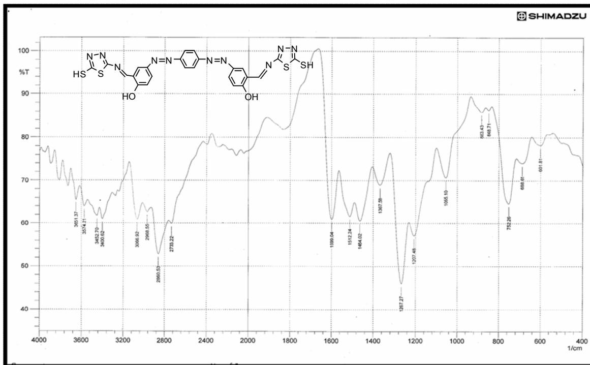
Fig. 3:FT-IR spectrum of compound [3]
