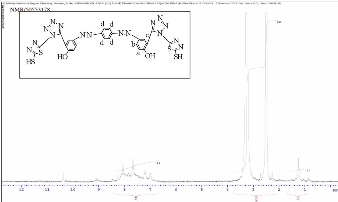
Fig .16: <sup>1</sup>H NMR spectrum of compound [8]
