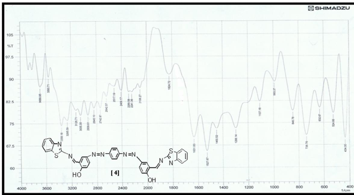
Fig. 4:FT-IR spectrum of compound [4]
