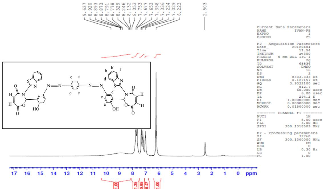
Fig .17: <sup>1</sup>H NMR spectrum of compound [9]
