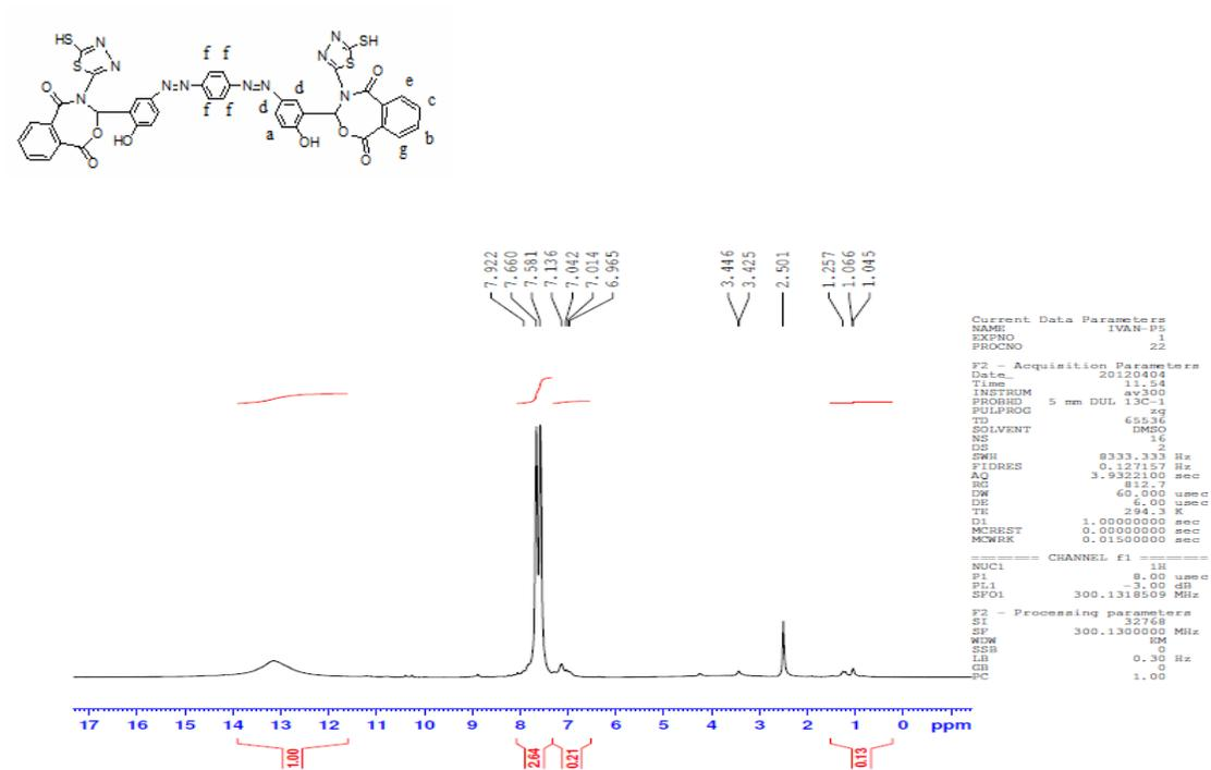
Fig . (14) : <sup>1</sup>H NMR spectrum of compound [6]
