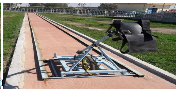
Figure (5) shows the installation of the railway and the movement of the device on it
