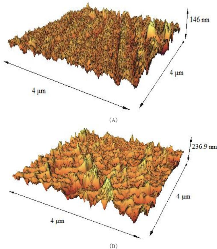
FIGURE (1) THE AFM OF (A) PS (B) Cu<sub>2</sub>O/PS
