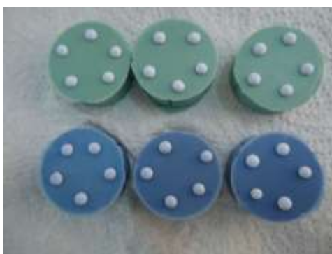
Figure (2):- Impression specimens with slurry droplets of dental stone.
