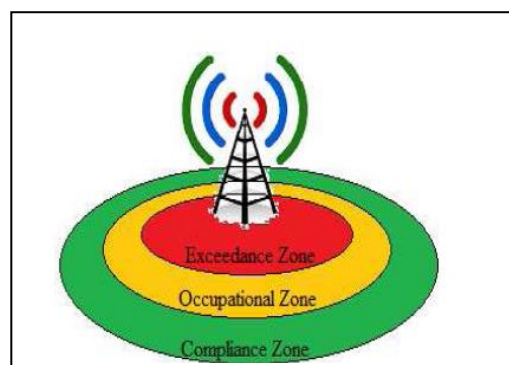
Fig. (5): Identification of zones around a base station antenna
