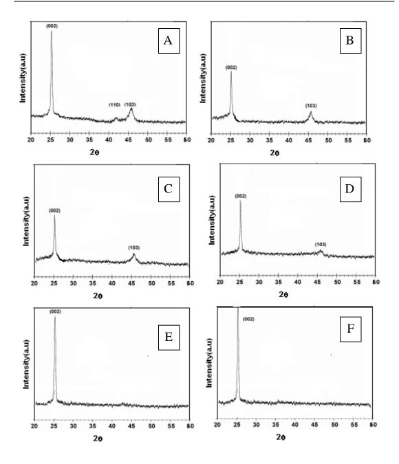
Fig.(1)X-ray diffraction for CdSe:Cu thin film for a- CdSe:Cu(5wt%)RT, CdSe:Cu (5wt%) at b-  $T_s=50$  °C, c-  $T_s=100$  °C, d-  $T_s=150$  °C, e-  $T_s=200$  °C, f-  $T_s=250$  °C
