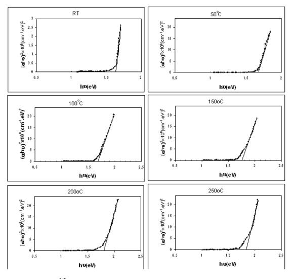
Fig.(3)The  $\alpha h v$ )<sup>1/2</sup> as a function of h v for CdSe:Cu thin films at different T<sub>s</sub>.
