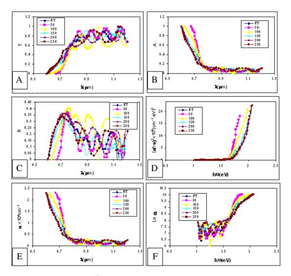
Fig.(2)The T, A, R,  $(\alpha h\nu)^{1/2}$ ,  $\alpha$  and  $\ln \alpha$  for CdSe:Cu thin films at different T<sub>s</sub>.
