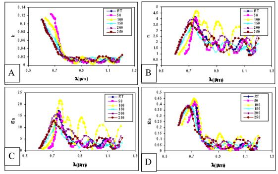
Fig.(4)The k,n,  $\varepsilon_1$  &  $\varepsilon_2$  as a function of  $\lambda$  for CdSe:Cu thin films at different T<sub>s</sub>.
