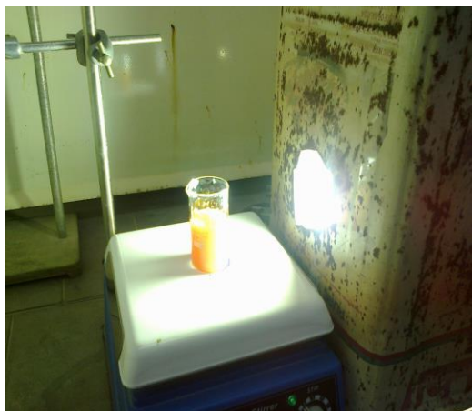
e) Image 1. UV-VIS illumination system using high pressure Hg lamp, 1000 watt
