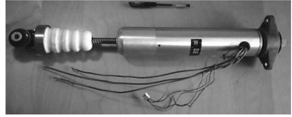
Fig. 3: Electromagnetic Actuator
