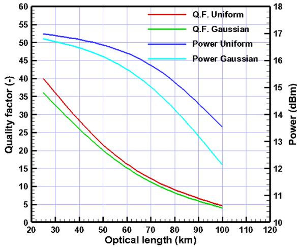
FIGURE 9. Q.F AND O/P POWER FOR UNIFORM WITH 8 MM FBG LENGTH
