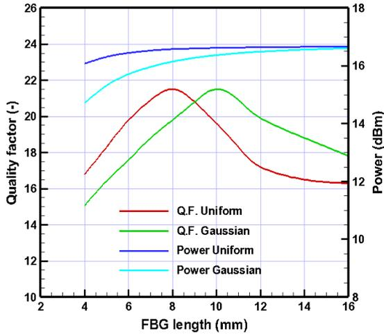
FIGURE 4. QUALITY FACTOR AND O/P POWER FOR UNIFORM AND GAUSSIAN CASES
