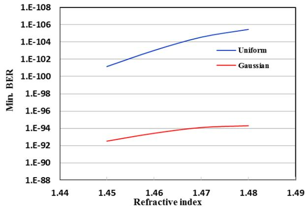
FIGURE 8. PERFORMANCE OF MIN. BER WITH REFRACTIVE INDEX FOR UNIFORM AND GAUSSIAN CASES
