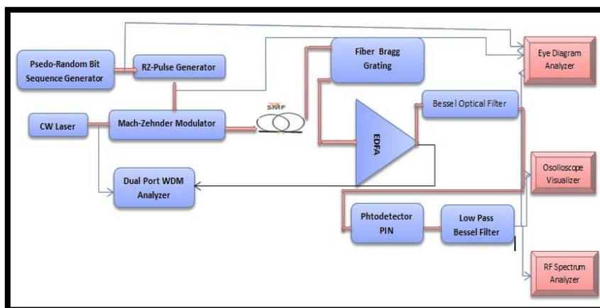
FIGURE 2. OPTISYSTEM SOFTWARE DIAGRAM OF THE DESIGNED AND SIMULATED MODEL OF THE MODULATOR
