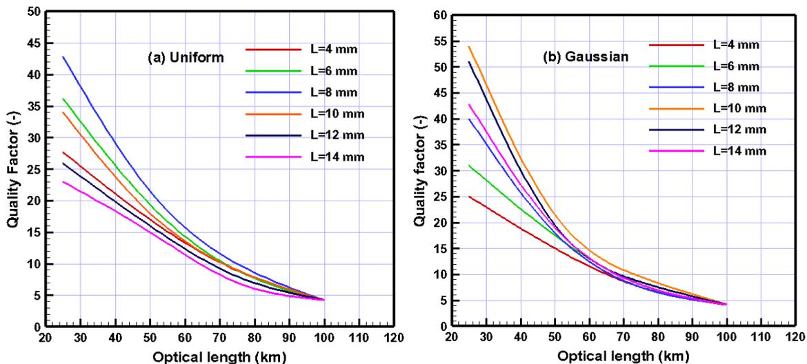
FIGURE 3 . SIX LENGTHS OF FBG ALONG THE OPTICAL CHANNEL THAT ARE TESTED TO GIVE MAXIMUM QF (A) UNIFORM CASE AND (B) GAUSSIAN CASE
