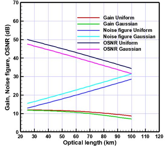
FIGURE 10. GAIN, N.F AND OSNR FOR UNIFORM AND GAUSSIAN CASES AND GAUSSIAN CASES WITH 8 MM FBG LENGTH
