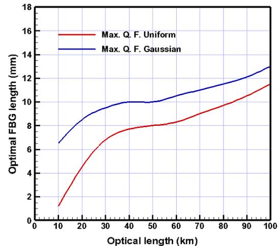
FIGURE 12 THE OPTIMAL FBG LENGTH WITH EACH POINT OF THE OPTICAL FIBER LENGTH
