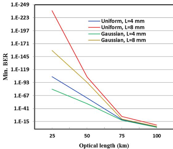
FIGURE 11 THE VARIATION OF THE MIN.BER WITH THE OPTICAL FIBER AT 8 MM FBG LENGTH
