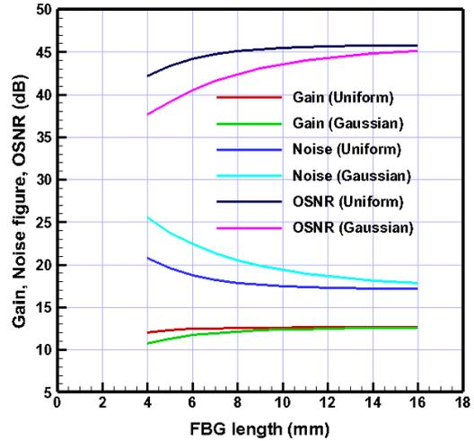
FIGURE 5. GAIN, NOISE FIGURE AND OSNR FOR UNIFORM AND GAUSSIAN CASES
