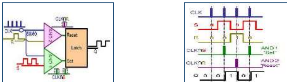
Fig. 3 Clocked SR flip-flop: (a) logic circuits; (b) working principle.
