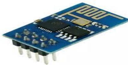
FIG. 7: ESP8266 MODULE
