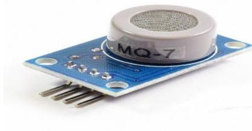
FIG. 2: MQ-7 GAS SENSOR
