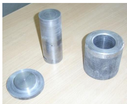
Fig.2. Manufactured Carbonate Steel Mold.
