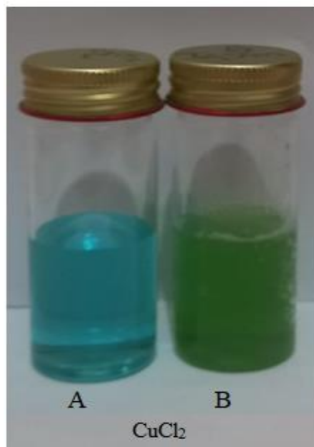
Figure (1) Color change of the fungal filtrate of A. carbonarius indicating the occurrence of biosynthesis of copper nanoparticles (A: copper chloride solution not treated with the fungal filtrate, B: copper chloride solution treated with the fungal filtrate)
