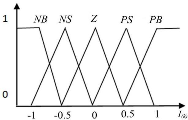
Fig. 7: Membership Function of input variables  $e$  and  $de$
