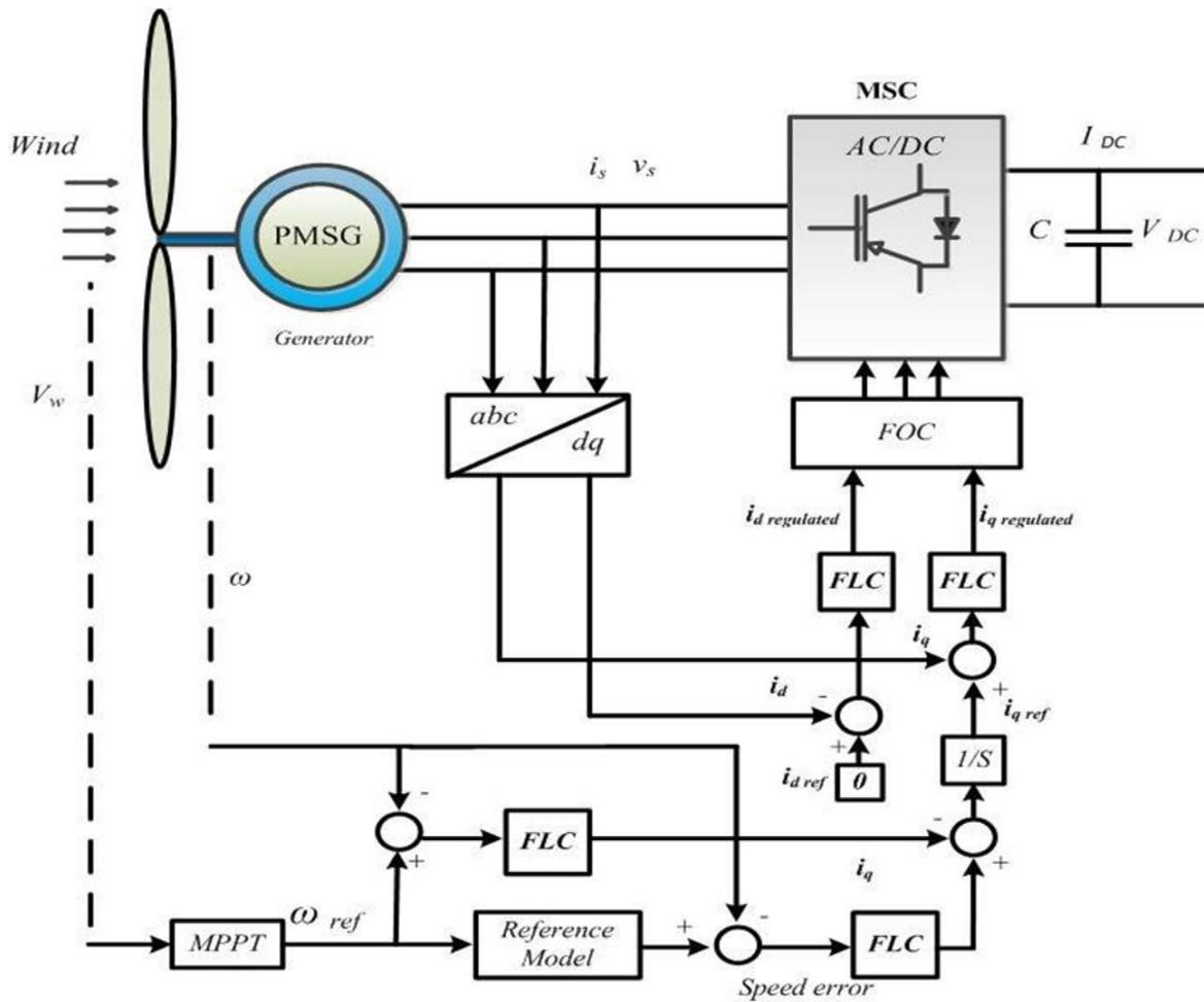
Fig. 6: MRFC - MSC Schematic Diagram
