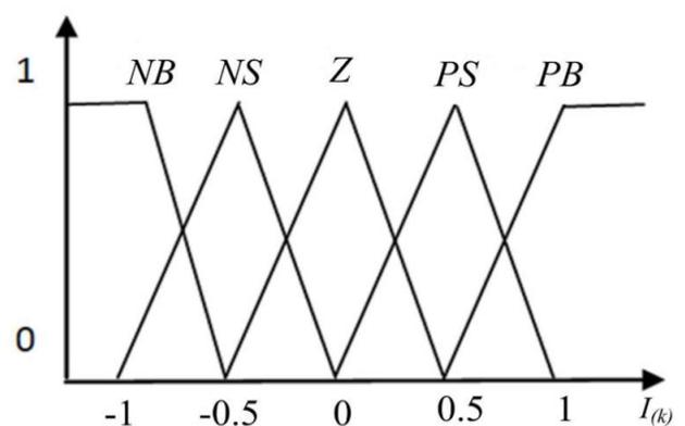
Fig. 8: Membership Function of output variables  $i_q$
