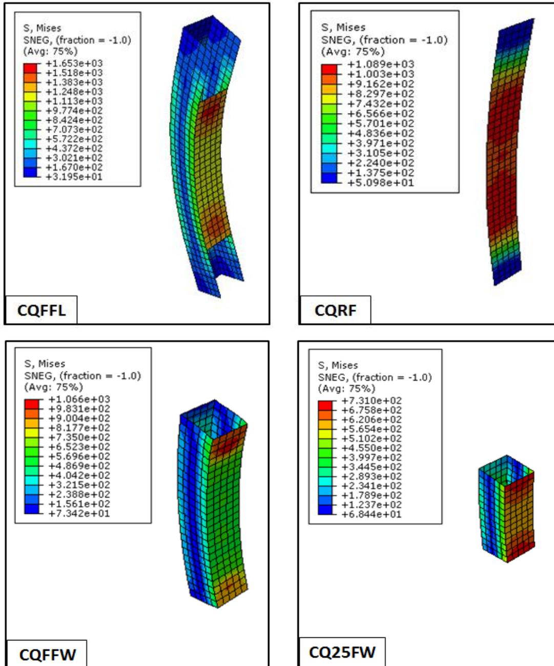
Figure 8. The distribution of the stress between CFRP laminate and concrete for specimens CQFFL, CQRF, CQFFW and CQ25FW.
