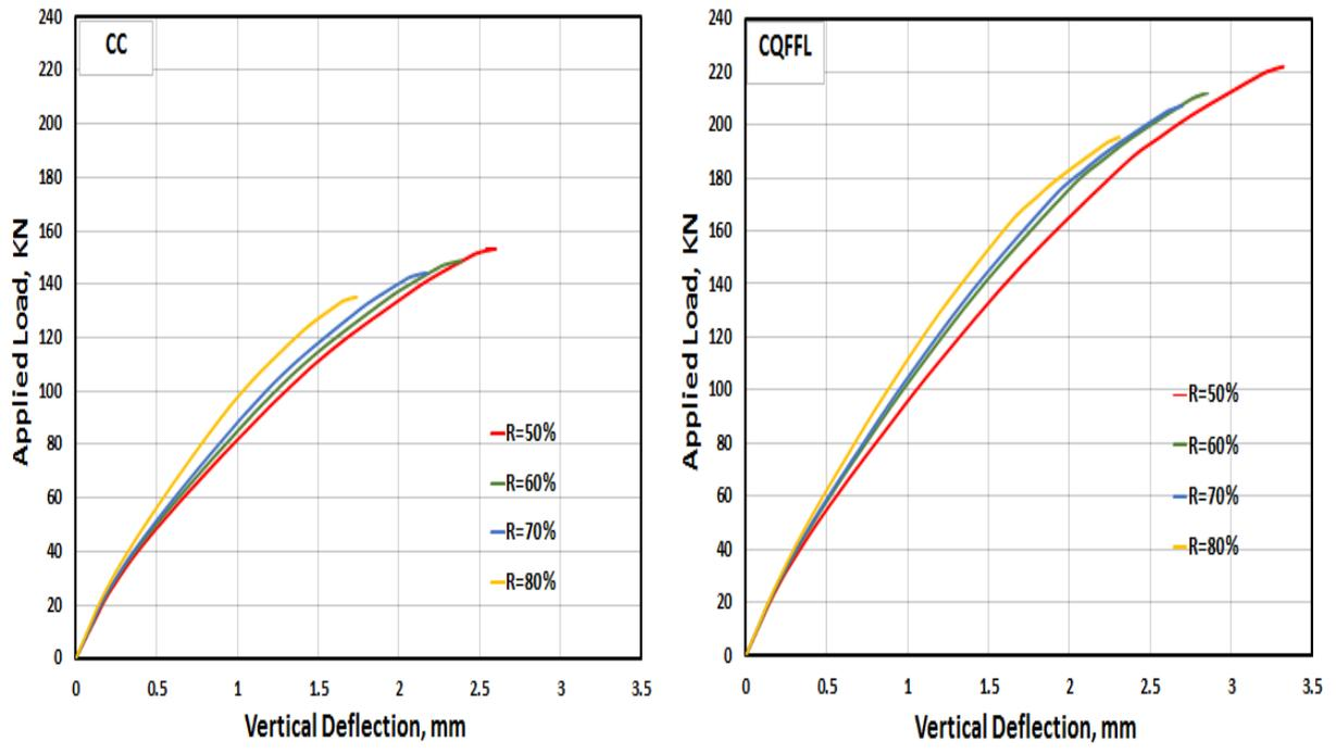
**Figure 11 Effect of change the initial load ratio for CC and CQFFL comparing with initial load ratio at 50% of the ultimate load.**
