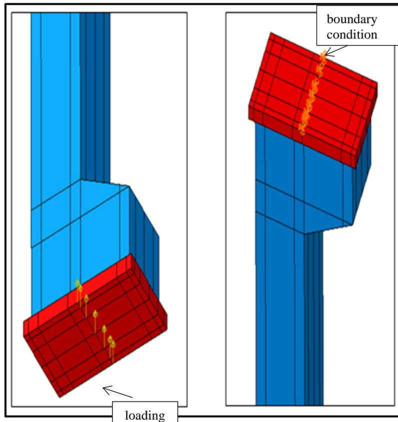
**Figure 3 Loading and boundary condition for the models**
