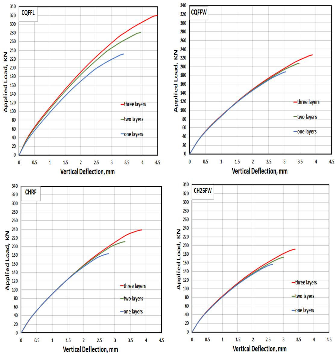
**Figure 9 Effect the number of layers for CQFFL, CQFFW, CHRf and CH25FW specimens**
