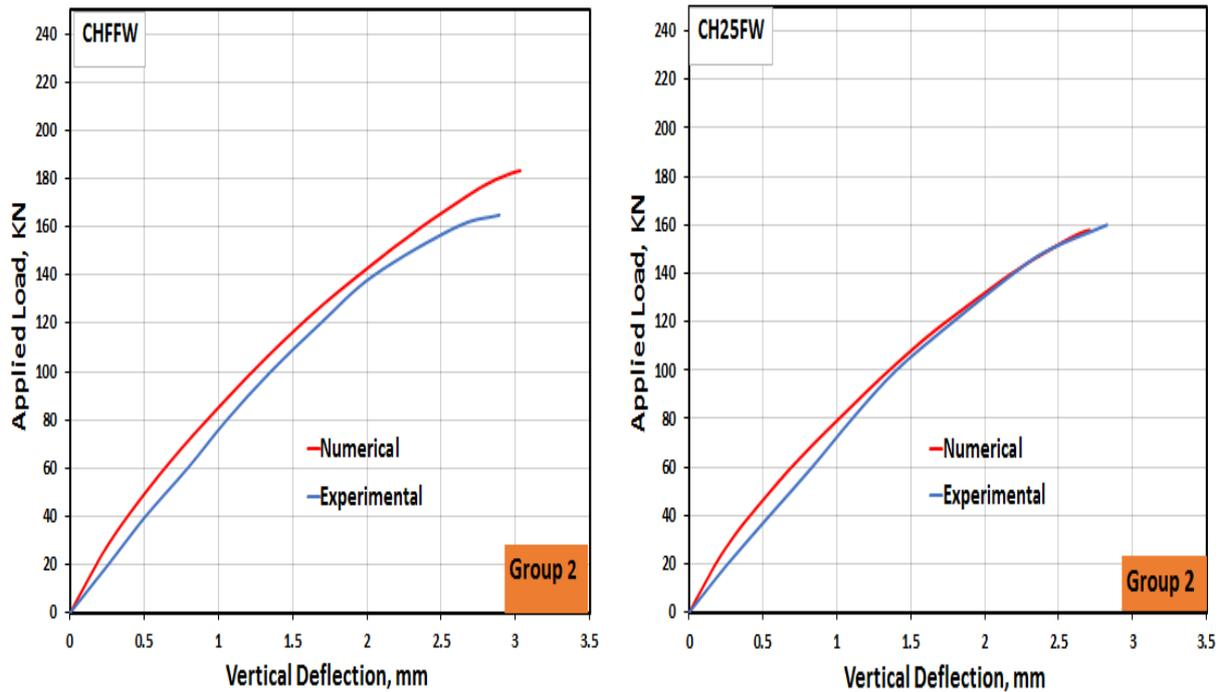
**Figure 6 The numerical and experimental curves for the columns**
