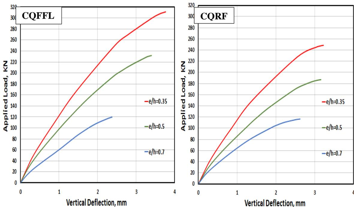
**Figure 10 Effect of various eccentricity load  $e/h$  for the load- vertical deflection curves for CQFFL and CQRF comparing with  $e/h=0.5$ .**
