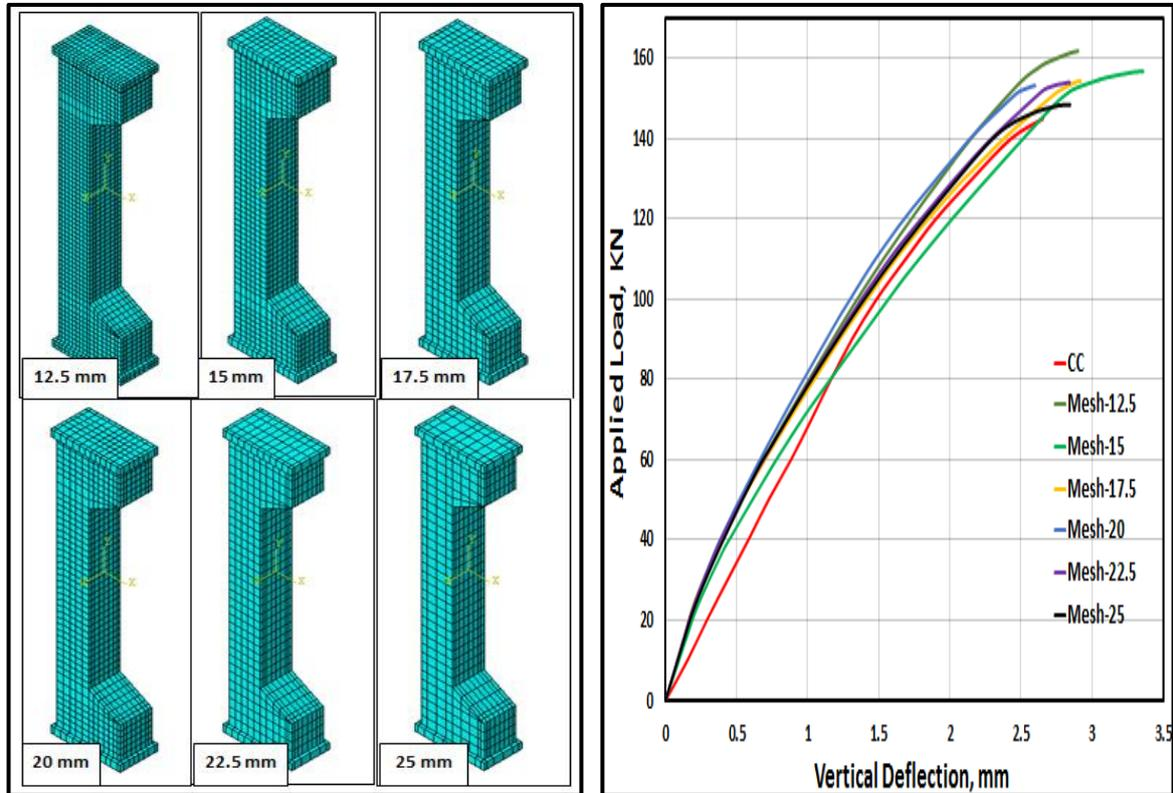
**Figure 5 (A) Finite element mesh density. (B) The impact of the element size on vertical load-deflection curves**
