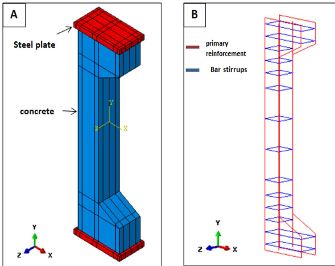
**Figure 1 The materials used (A) Concrete and steel plates (B) Steel reinforcement**
