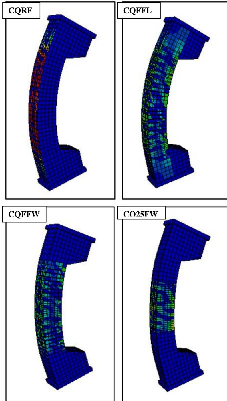
**Figure 7 Failure shapes of CFRP laminate for specimens CQFFL, CQRF, CQFFW and CQ25FW.**
