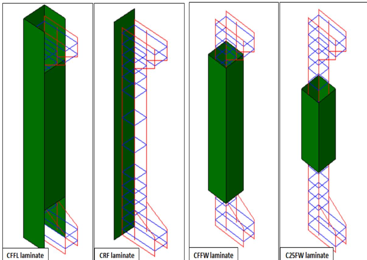
**Figure 2 CFRP laminate sizes arrangement**
