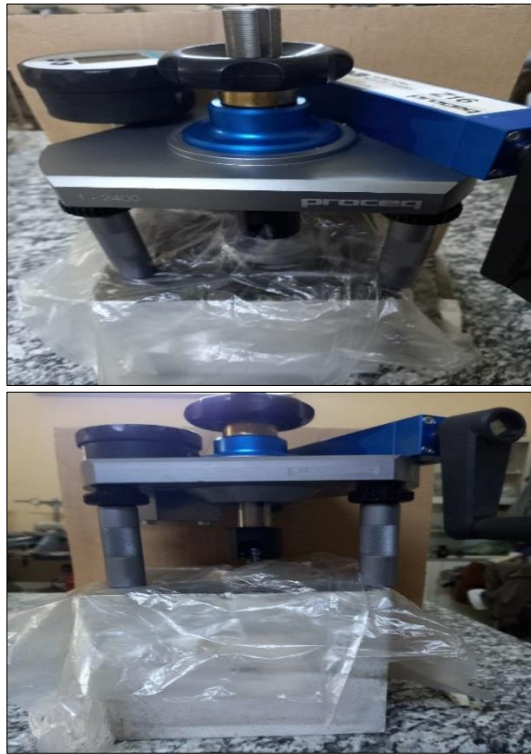
Figure (1): The Pull-off test
