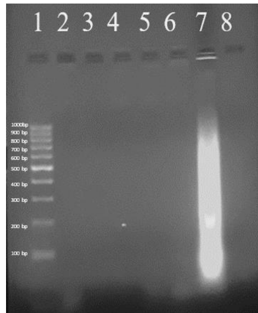
Figure 2: Extracted LPS of STEC in agarose gel (1: molecular weight marker, 2-6: ELPS, 7: bacterial suspension after sonicating and before DNase and RNase enzymes digestion, 8: negative control).
