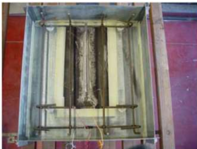
Fig. 11 Top view of this specimen CP1.1 before pouring the concrete [10] Supports
