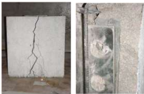
Fig. 14 Cracked slab and deformed perfobond rib at failure [10]
