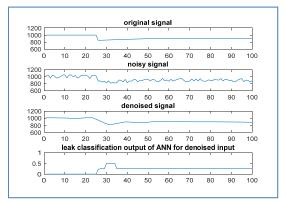
Fig. 6 Detection for  $0.25^{\prime\prime}$  leak
