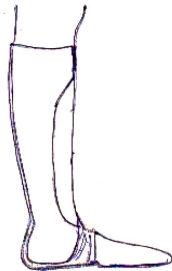
Figure (10): Sample of partial foot Prosthesis with \frac{2}{3} height between Knee joint axis & Ankle joint
