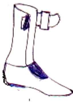
Figure (11): Sample of partial foot Prosthesis with \frac{1}{3} height between Knee joint axis & Ankle joint
