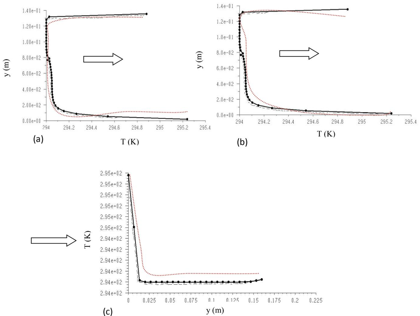
Figure (6) Temperature boundary layer profiles around the cubes at the vertical  $xy$  - plane at  $z=0.5\text{m}$ . (a) left surface ,(b) right surface ,(c) top surface. solid line with
