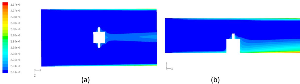
Figure (7) Contours of temperature distribution around the cube with VG.(a) the xz- plane at y=0.05m, (b) the xy-plane at z=0.25m.
