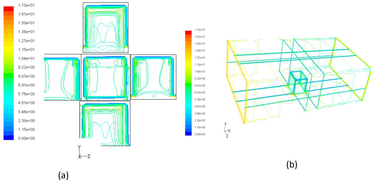
Figure (10) Contours of heat transfer coefficient ( $h$ ) without VG.(a) for the five faces of the cube,(b) for all faces of the cube.
