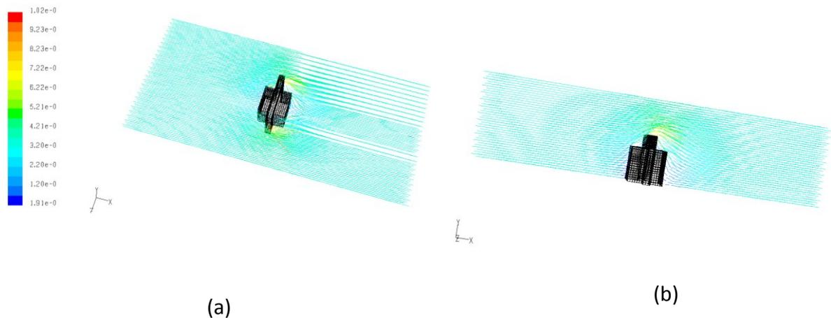
Figure (5) Time - a verged velocity vectors of the flow around the cube with VG.(a) the xz-plane at  $y=0.05m$  , (b)the xy-plane at  $z=0.25m$ .
