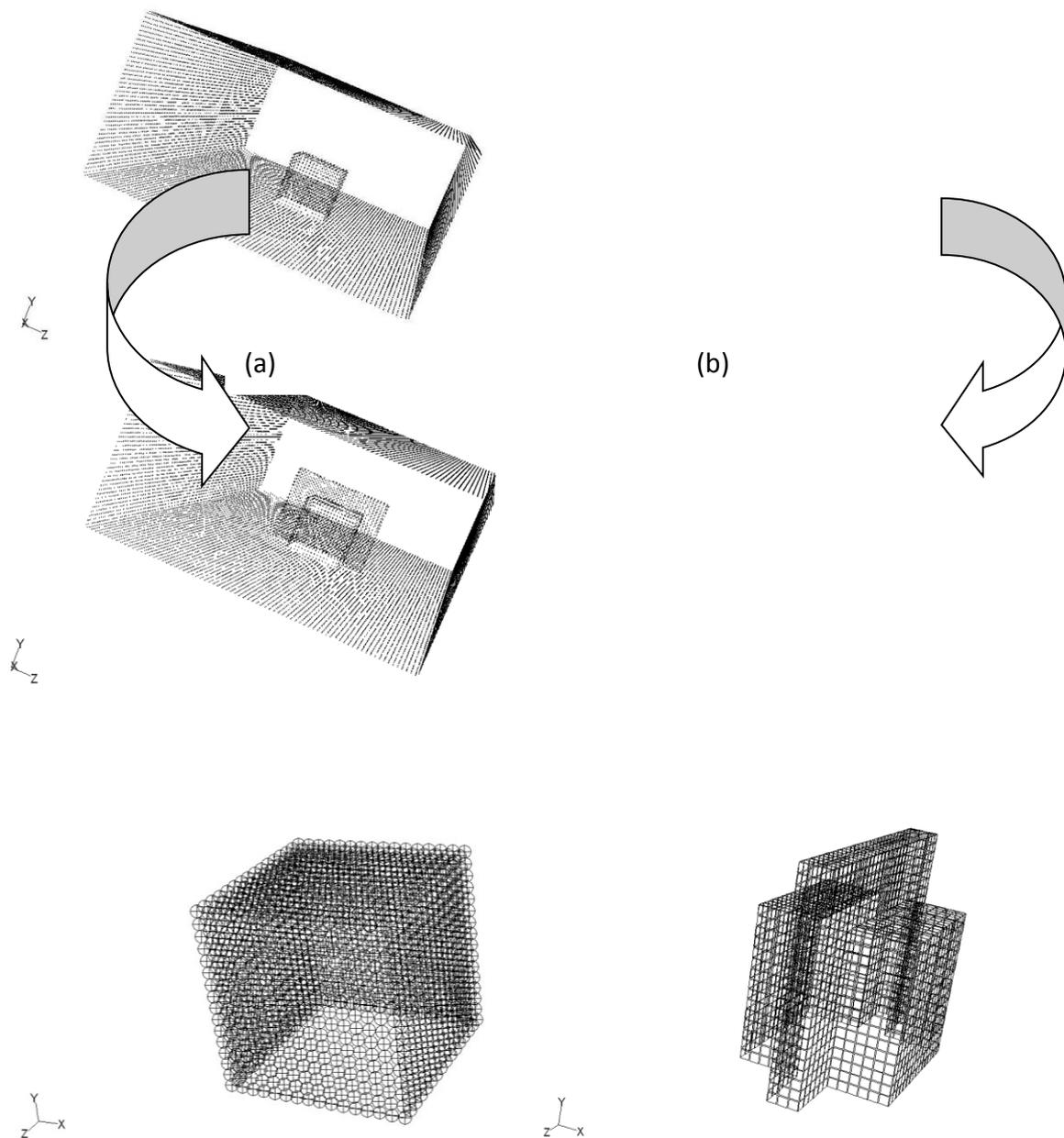
Figure (2) grid topology around cube.(a) without VG, (b)with VG.
