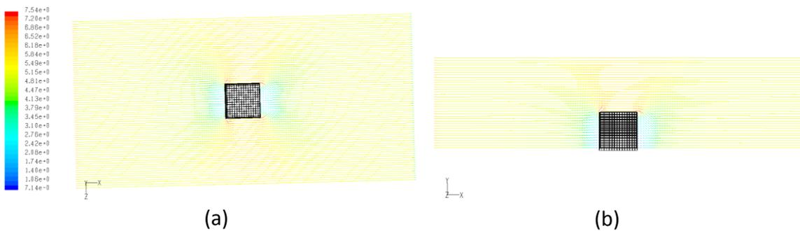
Figure (4 )Time - a verged velocity vectors of the flow around the cube without VG.(a) the xz-plane at  $y=0.05m$  , (b) the xy-plane at  $z=0.25m$ .
