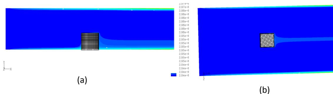
Figure (8) Contours of temperature distribution around the cube without VG.(a) the xz- plane at y=0.05m, (b) the xy-plane at z=0.25m.
