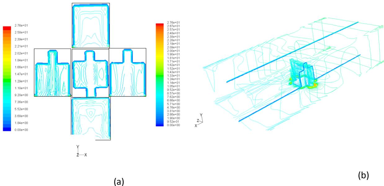
Figure (9) Contours of heat transfer coefficient ( $h$ ) with VG. (a) for the five faces of the cube,(b) for all faces of the cube.
