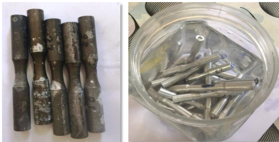
Figure 6: Container of 3.5% NaCl aqueous solution and samples after corroded by 3.5% NaCl
