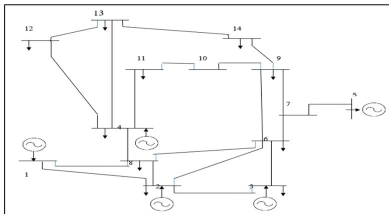
Figure 4: Single line diagram of IEEE 14-Bus system
