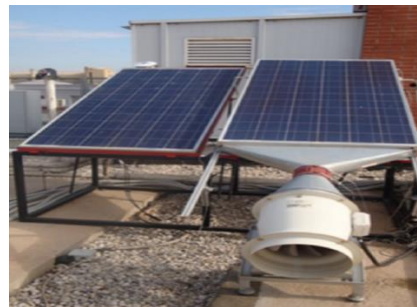
Figure 7: PV cooling by forced air.
