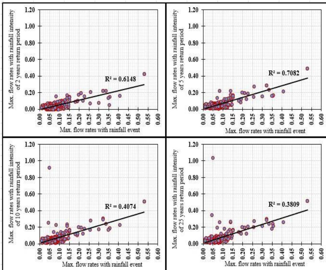
**Figure 4 Coefficient of determination ( $R^2$ ) between pipe flow rates obtained from the rainfall event modelling and rainfall intensity modelling for different return periods.**
