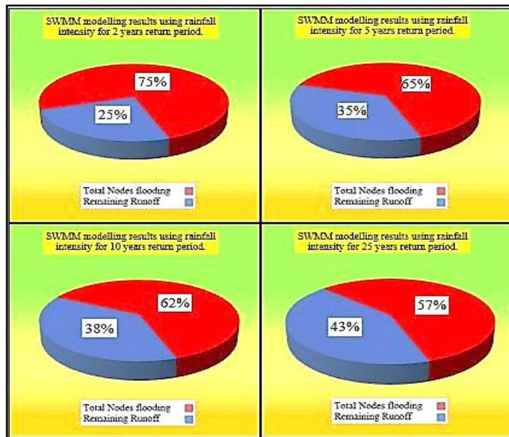
**Figure 5 Percentages of the total nodes flooding volume comparing with the remaining runoff volume in SWMM modelling.**
