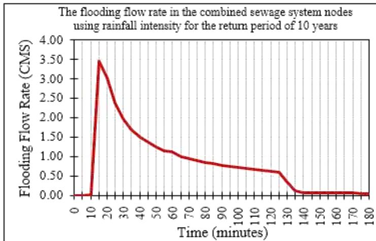
**Figure 8 The maximum flooding rate hydrographs from the SWMM modelling of the combined sewage system using the rainfall intensity for the return periods of 10 years.**
