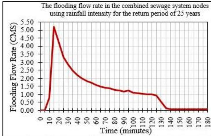
**Figure 9 The maximum flooding rate hydrographs from the SWMM modelling of the combined sewage system using the rainfall intensity for the return periods of 25 years.**
