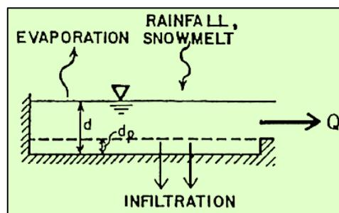
**Figure 3 Non-linear reservoir representation of sub-catchment in SWMM [24].**
