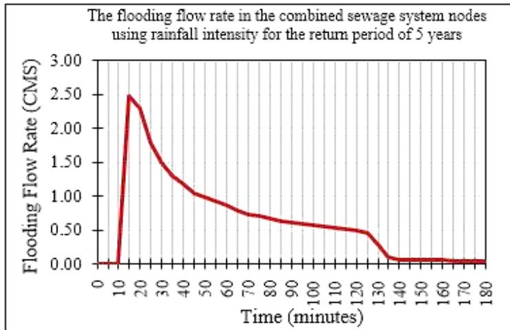
**Figure 7 The maximum flooding rate hydrographs from the SWMM modelling of the combined sewage system using the rainfall intensity for the return periods of 5 years.**
