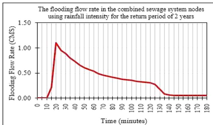
**Figure 6 The maximum flooding rate hydrographs from the SWMM modelling of the combined sewage system using the rainfall intensity for the return periods of 2 years.**
