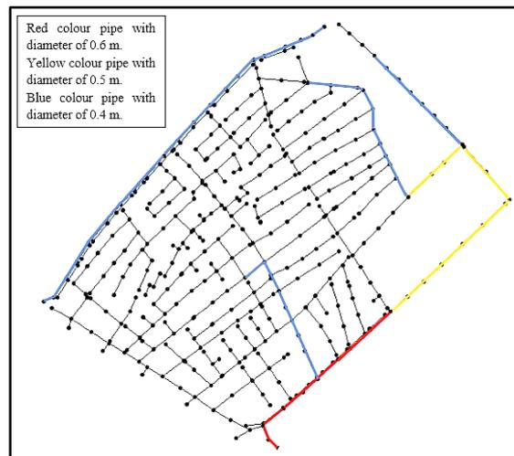
**Figure 11 The combined sewage system pipelines which diameters changed.**
