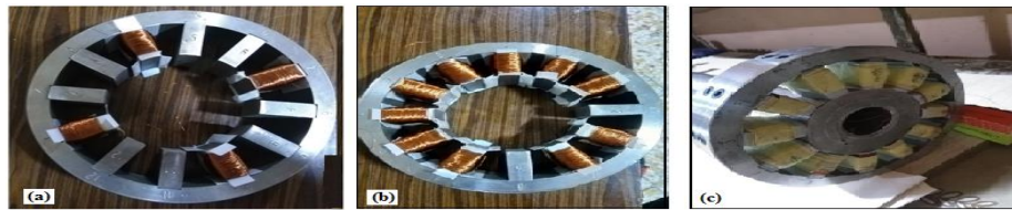
Figure 9: Steps of wrapping the poles
