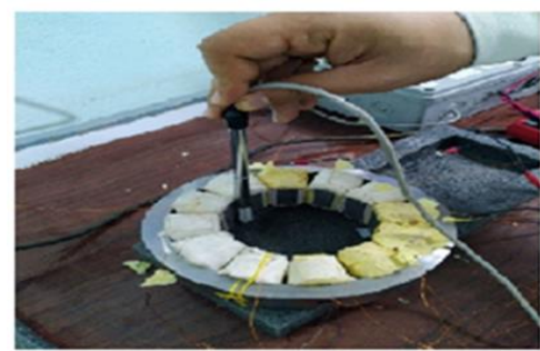
Figure 16: The position sensor for testing the magnetic density for each pole
