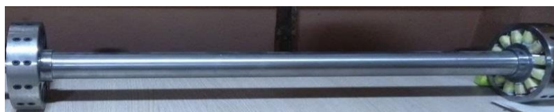
Figure 13: The rotor is made of metal type steel 37-2
