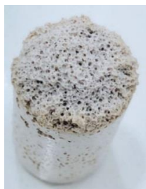
Figure 4: The specimen of geopolymer cement paste after curing 24 hr. at 25°C
