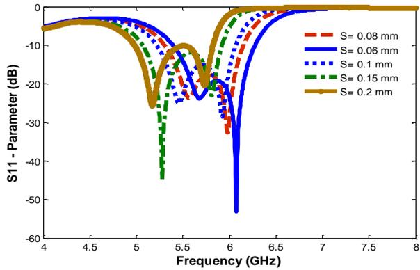
**Figure 9** The simulated  $S_{11}$ -parameter of the filtering antenna for various coupling spacing distances (S).
