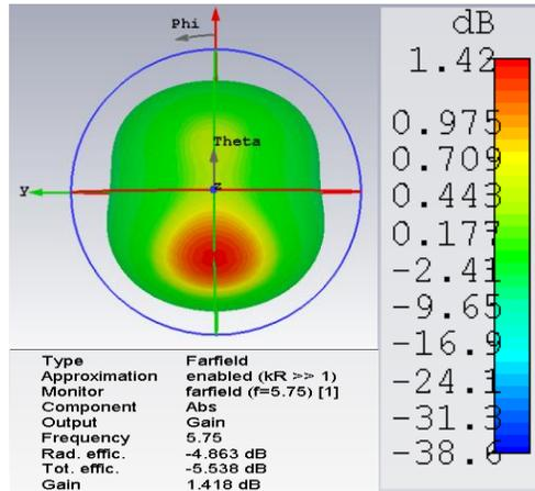
**Figure 3 The simulated radiation pattern of the rectangular patch antenna**
