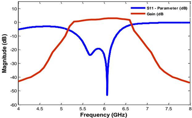
**Figure 8 Simulated  $S_{11}$  - Parameter gain of the optimized filtering antenna design.**
