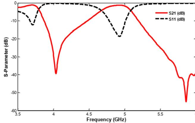
**Figure 6 Simulated S – parameter of the PCML – SIR**
