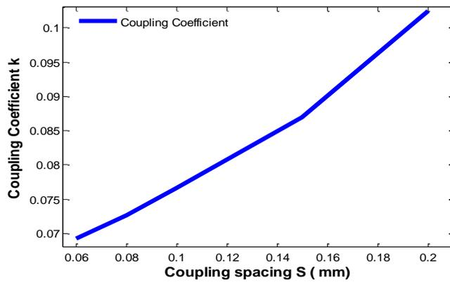
**Figure 10** The curve of the coupling coefficient changes with the coupling spacing S.
