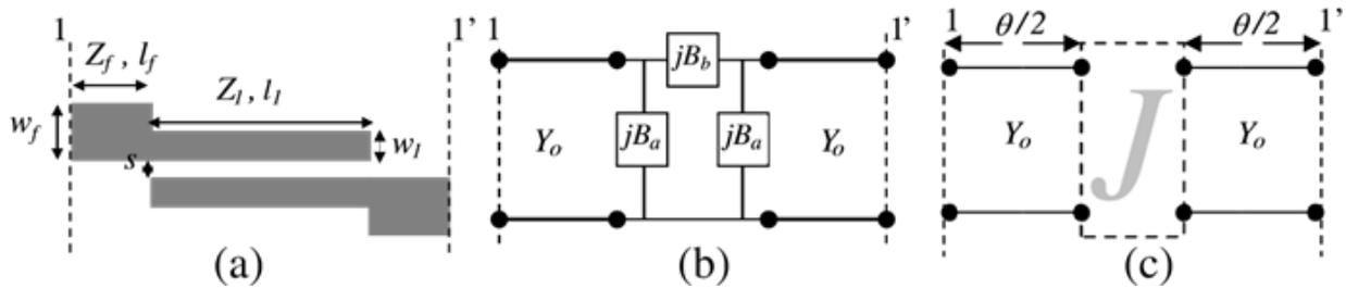
**Figure 4 (a) Single-stage of the PCML-SIR structure, (b) Equivalent circuit for reciprocal two-port network admittance for lossless PCML-SIR structure, (c) Equivalent J-inverter network with susceptance J of the PCML-SIR structure.**
