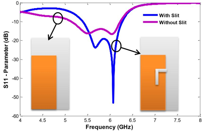
Figure 15 The  $S_{11}$  – parameter of the proposed filtering antenna with and
