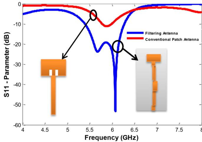
**Figure 12** The simulated  $S_{11}$ -parameter of the filtering antenna and the rectangular patch
