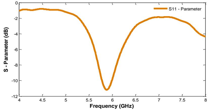
**Figure 2** Simulated  $S_{11}$ - parameter of the patch antenna design structure.
