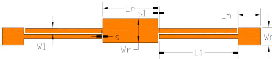
**Figure 5 PCML – SIR filter structure.**
