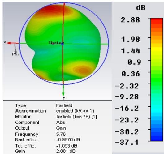
**Figure 13 Simulated results of the 3D far-field radiation pattern of the filtering antenna at 5.76 GHz.**
