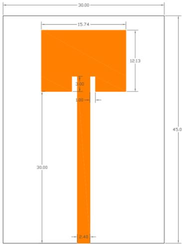
**Figure 1** The rectangular patch antenna.
