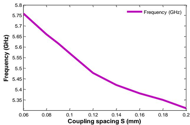
**Figure 11** The curve of the center frequency changes with the coupling spacing S.
