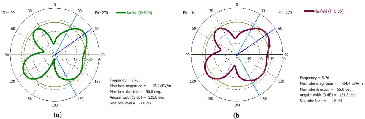
**Figure 14 Simulated far-field (a) E-field (b) H-field**
