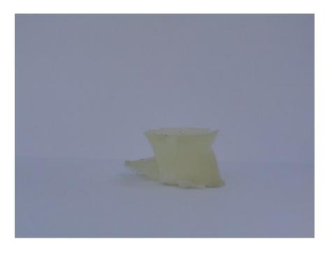
Fig.(5): Shape of failure of unreinforced epoxy specimen after compression test.
