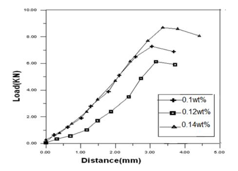
Fig.(8): data of compression test for epoxy specimens reinforced with PEG (0.1-0.14) wt %
