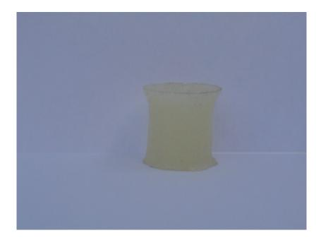
Fig.(6): Shape of failure of epoxy specimen reinforced with 0.12 wt % of CMC after compression test.
