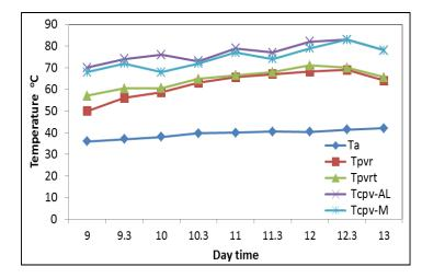
FIG. 4. VARIATION OF AMBIENT AND MODULE TEMPERATURES WITH DAY TIME
