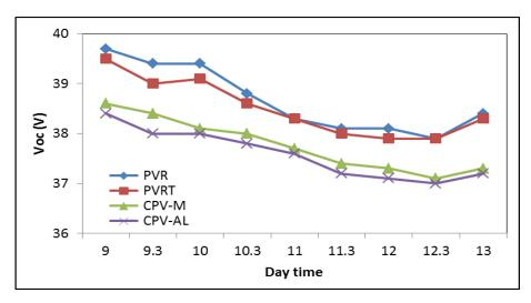
FIG. 5. PV SOLAR MODULE OPEN CIRCUIT VOLTAGE WITH DAY TIME.
