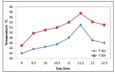
FIG. 3. Reflectors temperature versus day time
