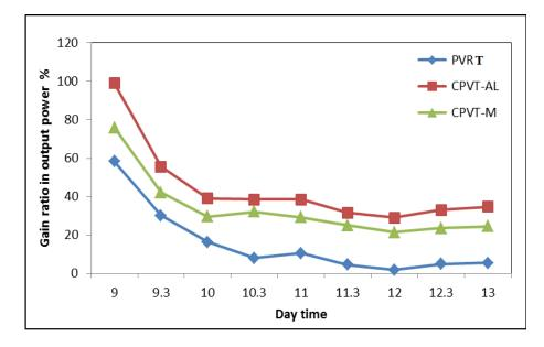
FIG. 8. GAIN RATIO IN OUTPUT POWER CPV MODULES IN COMPARE WITH FIXED REFERENCE MODULE.
